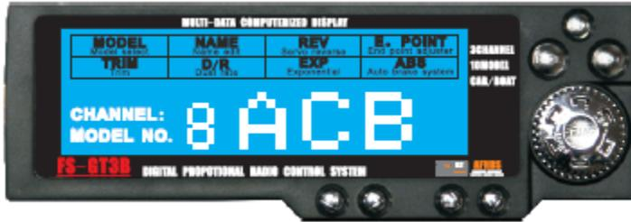
When the radio is initially turned on, it displays the current model number along with the name assigned to it. For reference the left digit (shown as 8 in the picture above) is referred to the number display and the 3 characters (shown as ACB) is referred to as the alphanumeric display.
